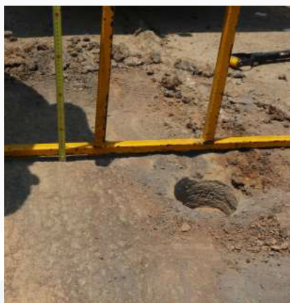
(17 January 2019) HVS test site after removal of the HVS showing less than 10 mm rut depth.
